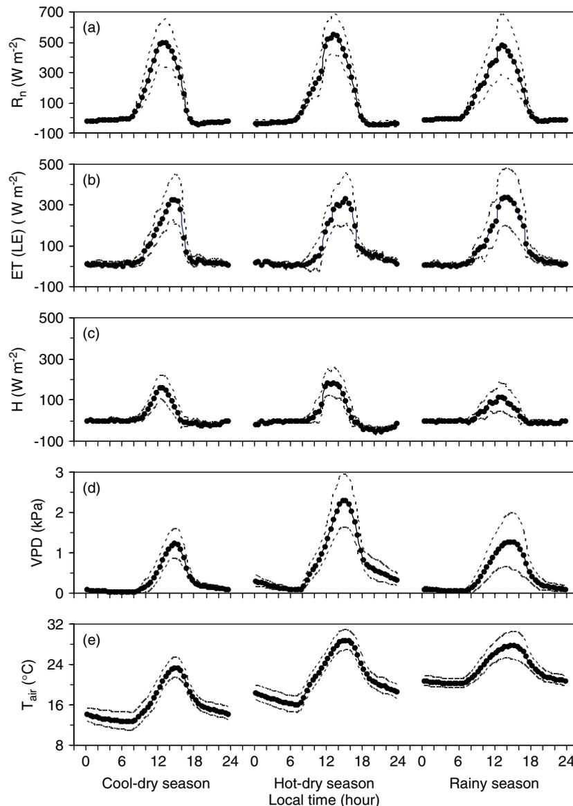
Figure 5. Diurnal variations of ecosystem ET (represented by latent heat flux), sensible heat flux ( $H$ ), net radiation ( $R_n$ ), water vapour pressure deficit (VPD) and air temperature ( $T_{\text{air}}$ ) in the cool-dry season, hot-dry season and rainy season. Solid circles are the means of all available 30-min data in each of the three seasons. Dash lines represent the SD of the 30-min data
