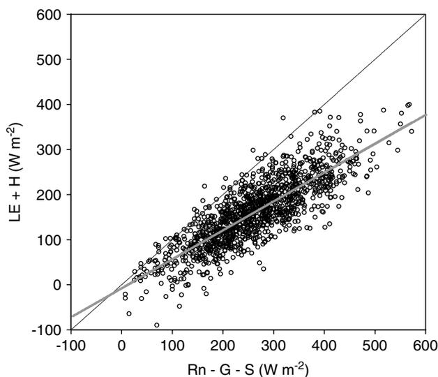
Figure 3. Relationship between the daily turbulent fluxes ( $LE + H$ ) measured by the eddy covariance system and available energy ( $R_n - G - S$ ) during the study period from 2003 to 2006 ( $y = 0.64x - 7.02$ ,  $r = 0.83$ ,  $n = 1219$ )
