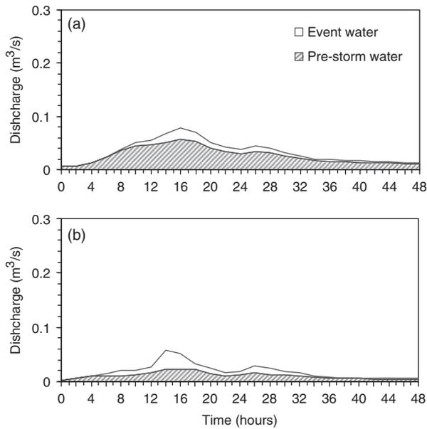
**Fig. 3.** Hydrograph separation of discharge into event water and pre-storm components from (a) the tropical seasonal rain forest and (b) the artificial rubber plantation catchment, 18–19 April 2004.
