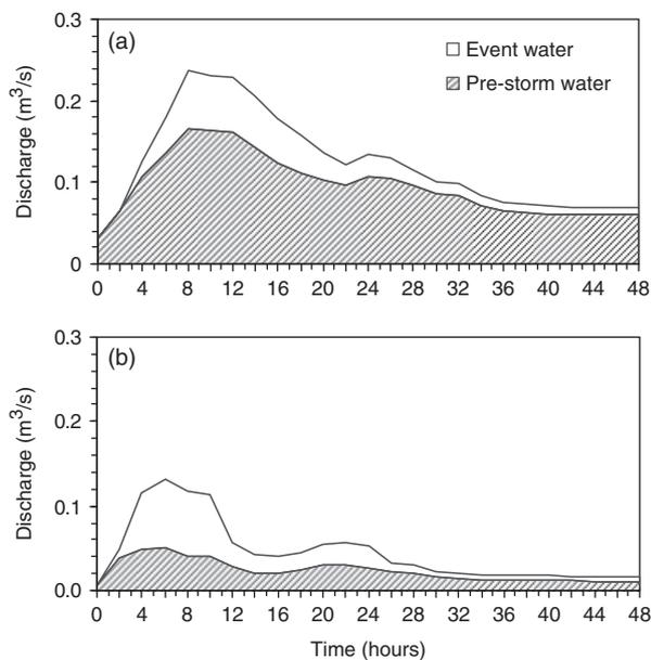
**Fig. 4.** Hydrograph separation of discharge into event water and pre-storm components from (a) the tropical seasonal rain forest and (b) the artificial rubber plantation catchment, 8–9 September 2004.
